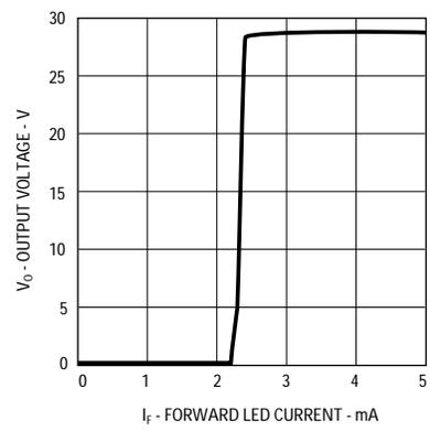
Figure 15. Transfer Characteristics
