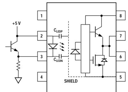
Figure 32. Recommended LED Drive Circuit for Ultra-High CMR
