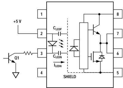
Figure 31. Not Recommended Open Collector Drive Circuit
