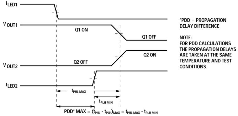
Figure 33. Minimum LED Skew for Zero Dead Time
