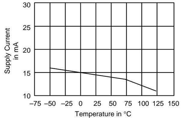
**Figure 2. Typical Supply Current vs. Temperature**
