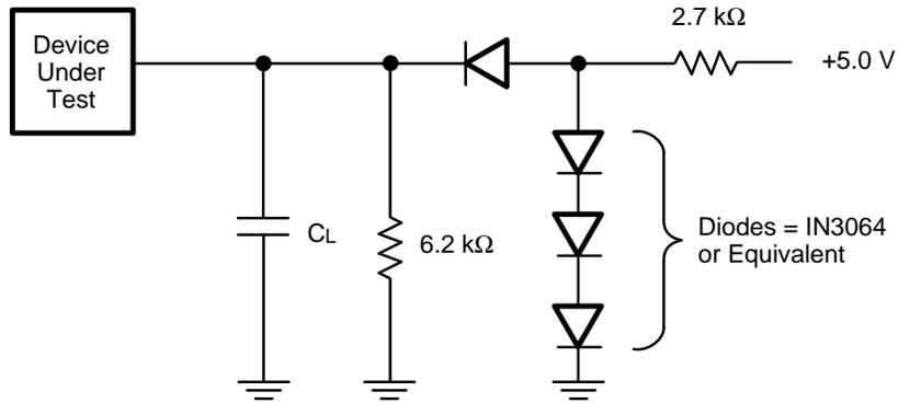
$C_L = 100 \text{ pF}$  including jig capacitance (30 pF for -55, -70)
