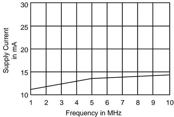
**Figure 1. Typical Supply Current vs. Frequency**
