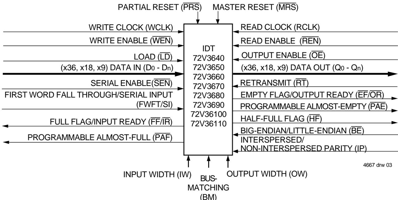
Figure 1. Single Device Configuration Signal Flow Diagram
