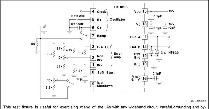
This test fixture is useful for exercising many of the UC1825's functions and measuring their specifications.
