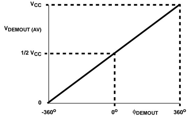
**FIGURE 4. PHASE COMPARATOR 2: AVERAGE OUTPUT VOLTAGE vs INPUT PHASE DIFFERENCE:**
