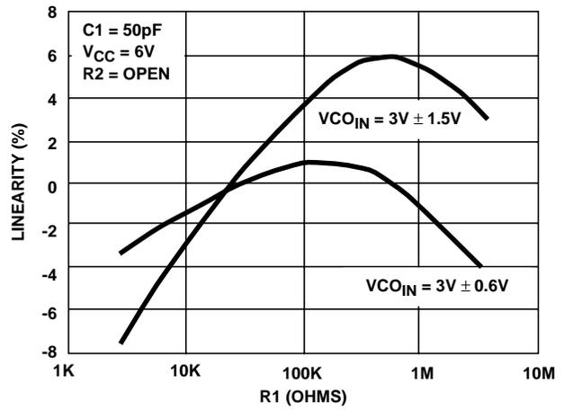
FIGURE 36. HC4046A VCO LINEARITY vs R1 ( $V_{CC} = 6V$ )
