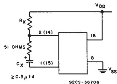
Fig. 18 - Alternate rapid power-down protection circuit.
