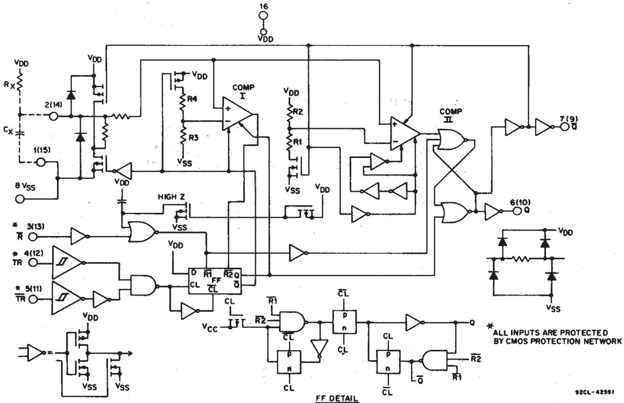
Fig. 1 - Logic diagram (1/2 of device shown).
