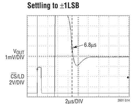
$V_{CC} = 5V$ ,  $V_{REF} = 4.096V$
