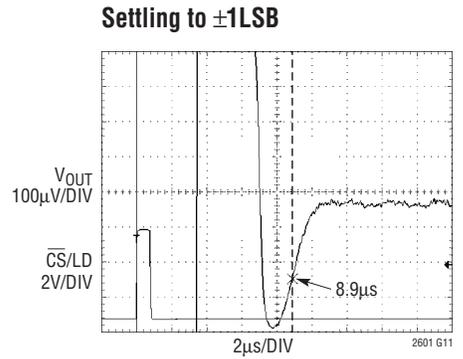
$V_{CC} = 5V$ ,  $V_{REF} = 4.096V$
