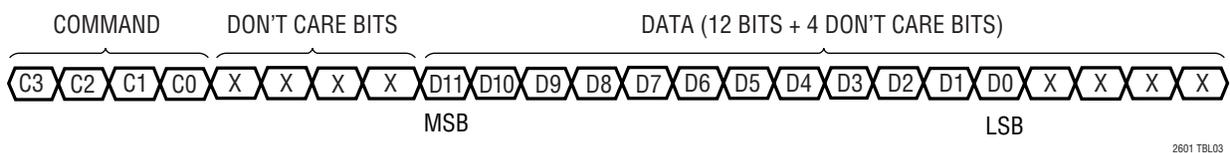
Because of this, the devices can be addressed and controlled individually by simply concatenating their input words; the first instruction addresses the last device in the chain and so forth. The SCK and  $\overline{\text{CS/LD}}$  signals are common to all devices in the series.
