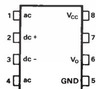
The connection of a 0.1  $\mu$ F bypass capacitor between pins 8 and 5 is recommended.
