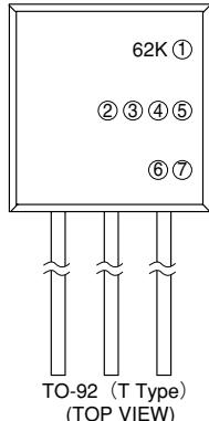
① Represents the Polarity of Output Voltage
