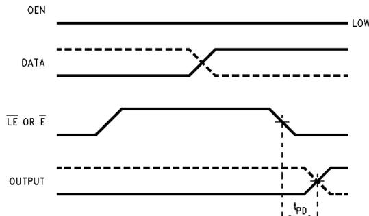
FIGURE 4. Propagation Delay LE, E to Q
