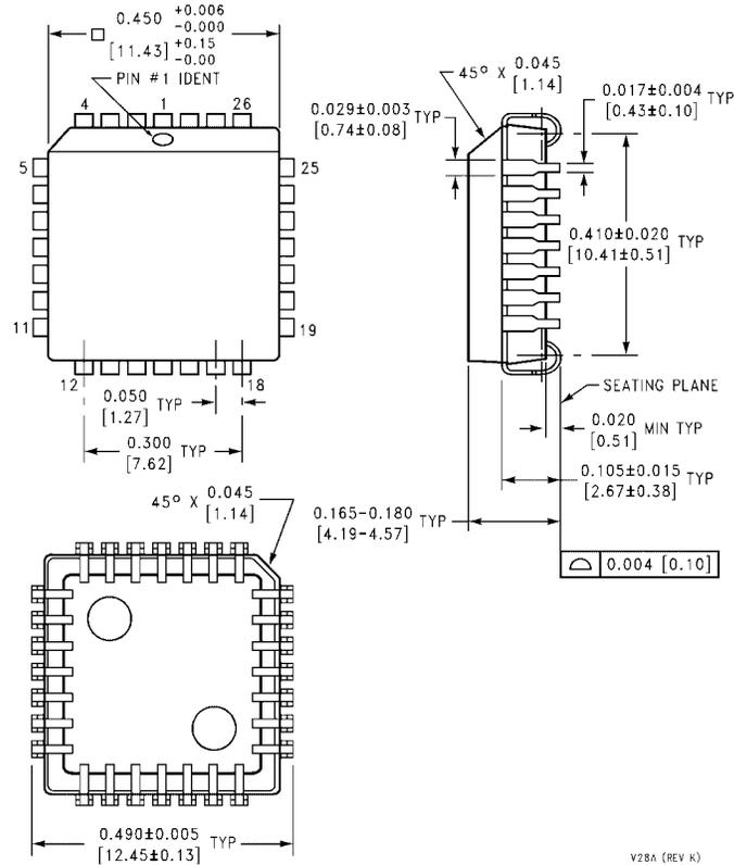
**28-Lead Plastic Lead Chip Carrier (PLCC), JEDEC MO-047, 0.450 Square
