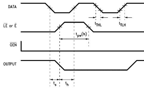
FIGURE 3. Setup, Hold and Pulse Width Times
