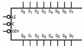
100344 Low Power 8-Bit Latch with Cut-Off Drivers
