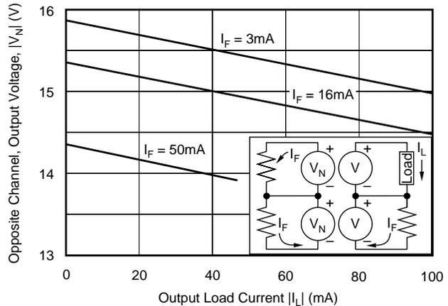
NOTES: (1) Using a 104mm x 19mm x 1.6mm aluminum strip mounted to the bottom of the case with heat sink compound. (2) Total output current is the sum of the currents for each individual output.
