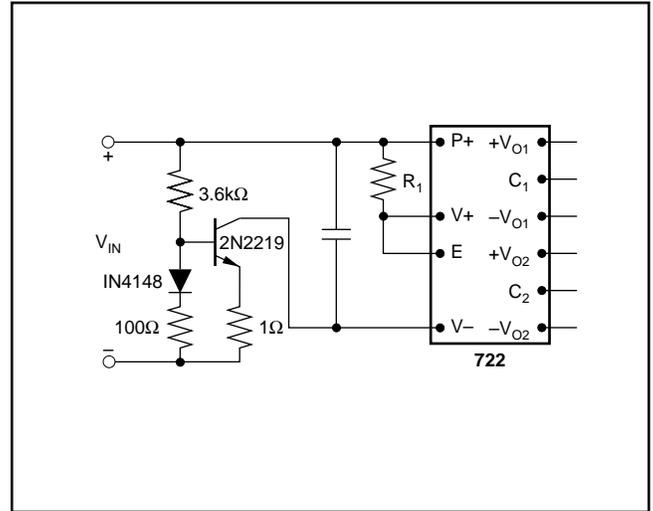
FIGURE 3. Short-Circuit Protection.
