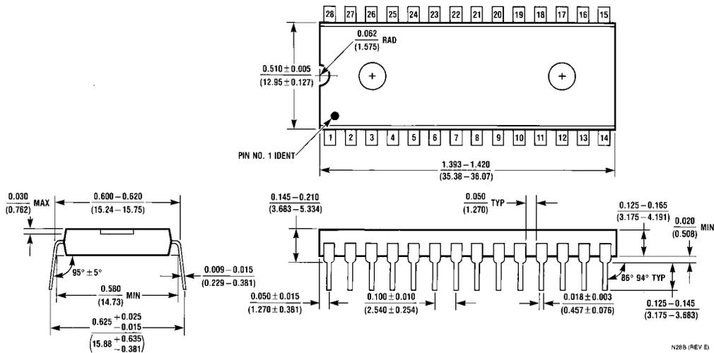
**28-Lead Plastic Dual-In-Line Package (PDIP), JEDEC MS-010, 0.600" Wide
