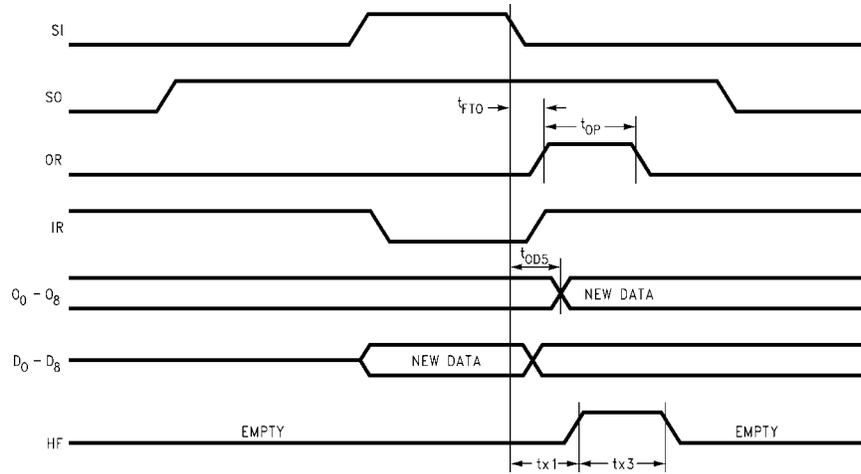
**Note:** FULL is LOW;  $\overline{MR}$  is HIGH;  $\overline{OE}$  is LOW;  $t_{DOF} = t_{FTO} - t_{OD5}$ . Data output transition—valid data arrives at output stage  $t_{DOF}$  after OR is HIGH.
