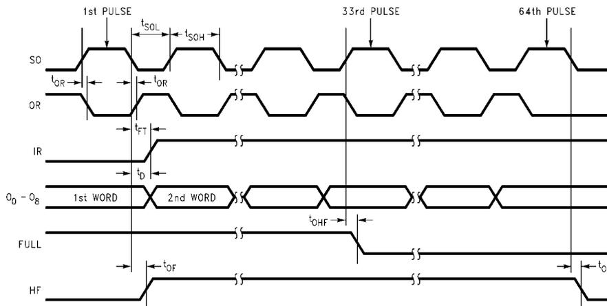
Note:  $\overline{SI}$  and  $\overline{OE}$  are LOW;  $\overline{MR}$  is HIGH;  $D_0 - D_8$  are immaterial.
