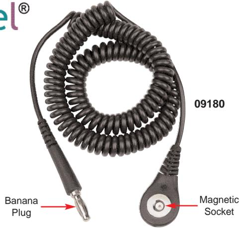
Jewel® MagSnap Coil Cords meet or exceed the requirements of ANSI/ESD S20.20 and ANSI/ESD S1.1 including section 5.4 Breakaway Force "With the ground cord connected to the cuff in a normal manner, a force of  $\geq .45$  kg (1 lb) but  $\leq 2.3$  kg (5 lb) applied to the ground cord, in the normal disconnect direction, shall be required to separate the ground cord from the cuff."
