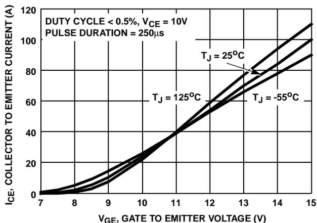
FIGURE 13. TRANSFER CHARACTERISTIC
