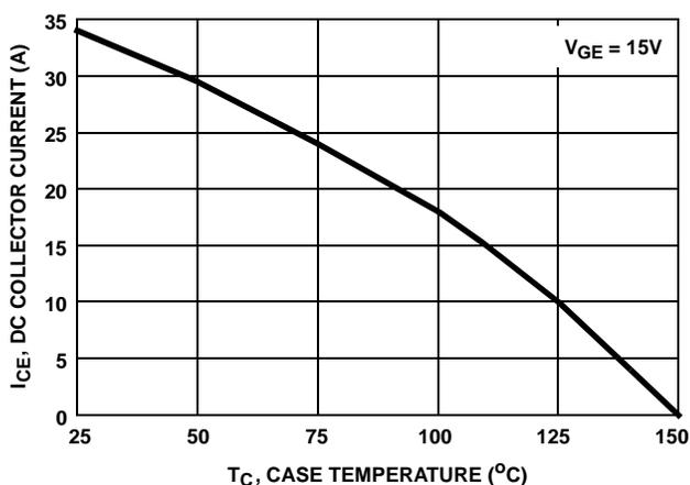
FIGURE 1. DC COLLECTOR CURRENT vs CASE TEMPERATURE
