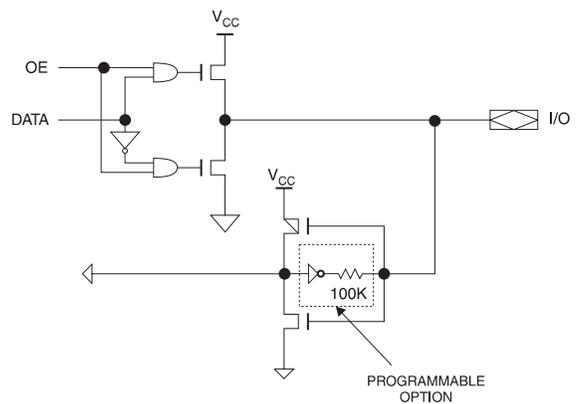
To further reduce power, each ATF1504AS macrocell has a Reduced Power bit feature. This feature allows individual macrocells to be configured for maximum power savings. This feature may be selected as a design option.
