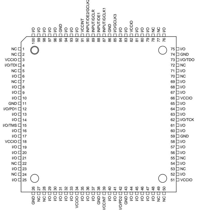
TTL, SSI, MSI, LSI and classic PLDs. The ATF1504AS's enhanced routing switch matrices increase usable gate count, and the odds of successful pin-locked design modifications.
