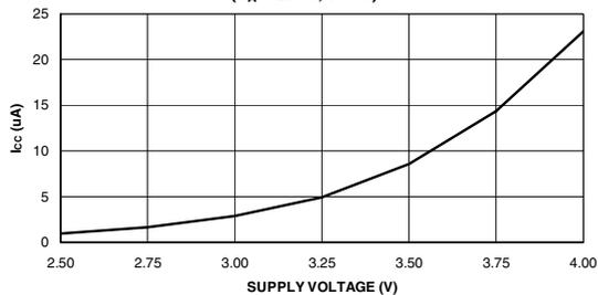
**OUTPUT SINK CURRENT VS. SUPPLY VOLTAGE**
