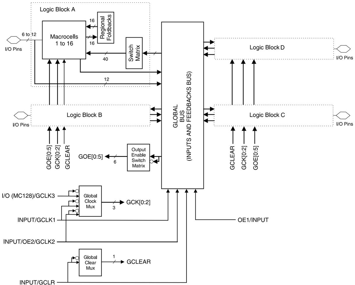
Unused product terms are automatically disabled by the compiler to decrease power consumption. A security fuse, when programmed, protects the contents of the ATF1504ASV(L). Two bytes (16 bits) of User Signature are accessible to the user for purposes such as storing project name, part number, revision or date. The User Signature is accessible regardless of the state of the security fuse.
