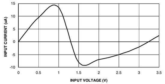
**INPUT CLAMP CURRENT VS. INPUT VOLTAGE**
