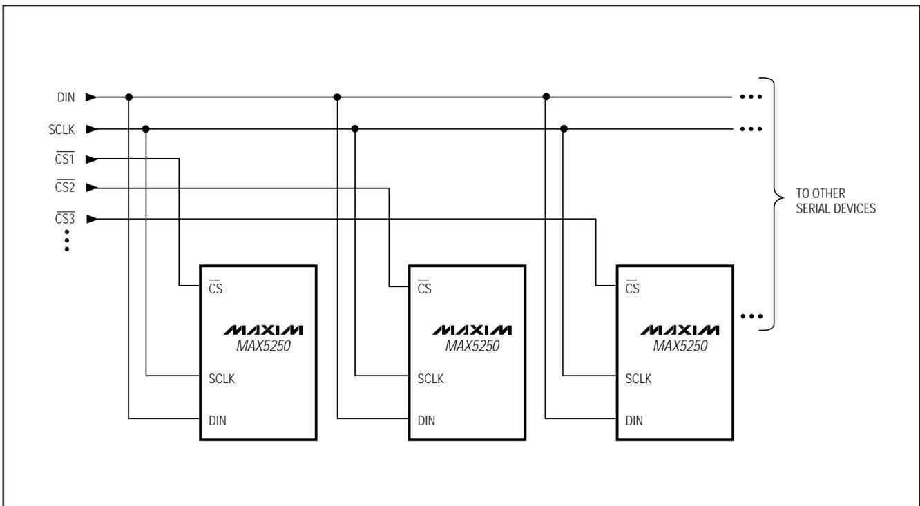
Figure 8. Multiple MAX5250s Sharing a Common DIN Line
