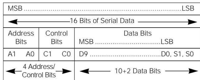
Figure 4. Serial-Data Format
