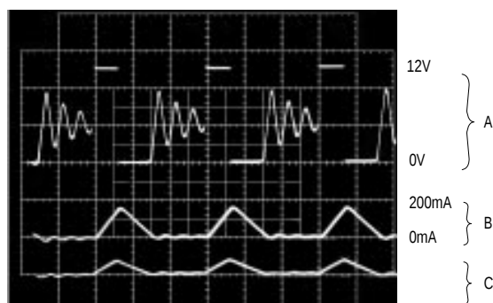
MAX738A/MAX744A SWITCHING WAVEFORMS, DISCONTINUOUS CONDITION
