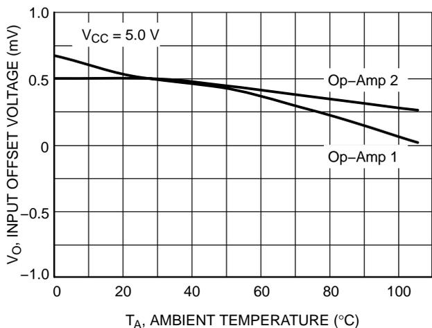
**Figure 6. Input Offset Voltage vs. Ambient Temperature**
