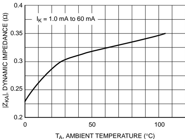
**Figure 4. Reference Dynamic Impedance vs. Ambient Temperature**
