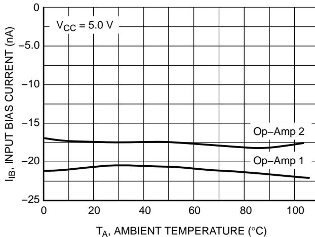
**Figure 7. Input Bias Current vs. Ambient Temperature**
