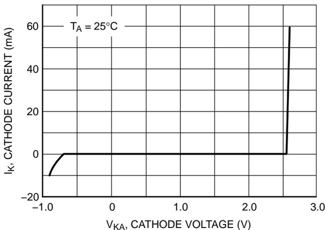
**Figure 2. Reference Cathode Current vs. Cathode Voltage**
