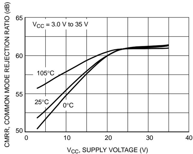
**Figure 8. Common Mode Rejection Ratio vs. Supply Voltage**
