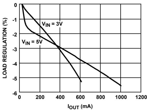
FIGURE 5. V<sub>BOOST</sub> LOAD REGULATION (P MODE)
