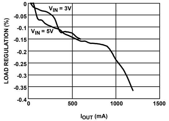
FIGURE 4. V<sub>BOOST</sub> LOAD REGULATION (PI MODE)
