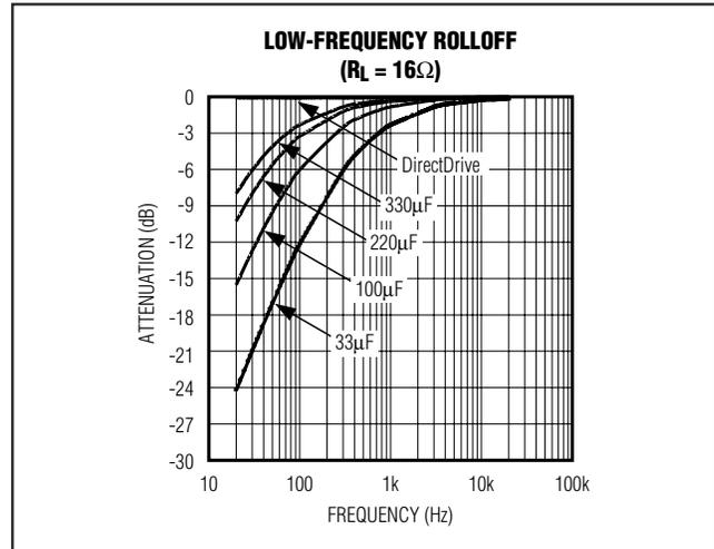
Figure 3. Low-Frequency Attenuation of Common DC-Blocking Capacitor Values
