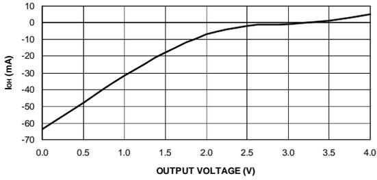
**OUTPUT SINK CURRENT VS. OUTPUT VOLTAGE**
