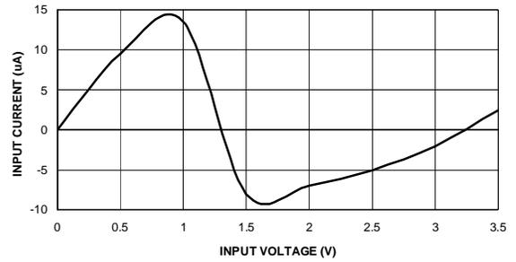
**INPUT CLAMP CURRENT VS. INPUT VOLTAGE**
