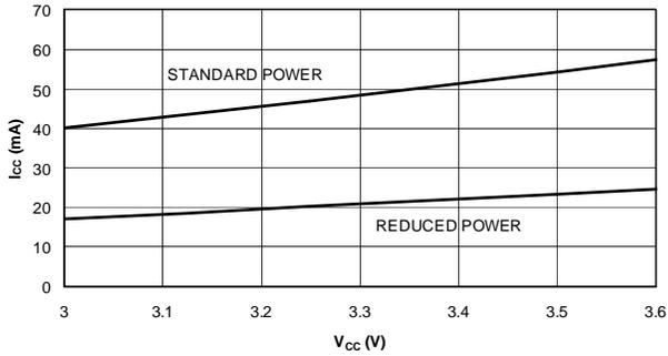
**OUTPUT SOURCE CURRENT VS. SUPPLY VOLTAGE**
