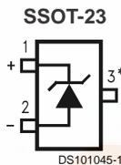
\*This pin must be left floating or connected to pin 2.
