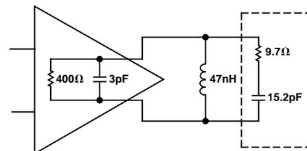
Figure 8. Saw Filter Model (170 MHz)
