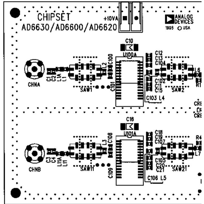
Figure 12. Reference Design Component Placement (Two Channels Shown)
