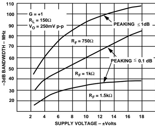
Figure 23. Bandwidth vs. Supply Voltage, Gain = +1,  $R_L = 150\ \Omega$
