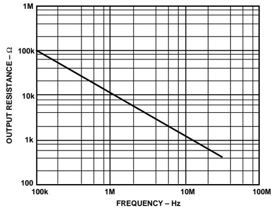
Figure 10. Output Resistance vs. Frequency, Disabled State
