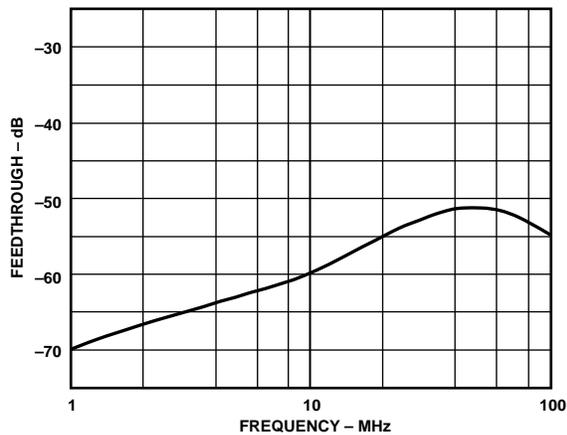
Figure 57. 4:1 Mux OFF Channel Feedthrough vs. Frequency
