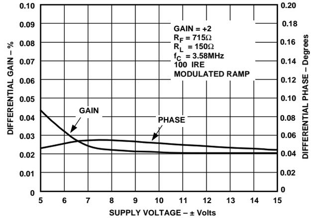
Figure 49. Differential Gain and Phase vs. Supply Voltage
