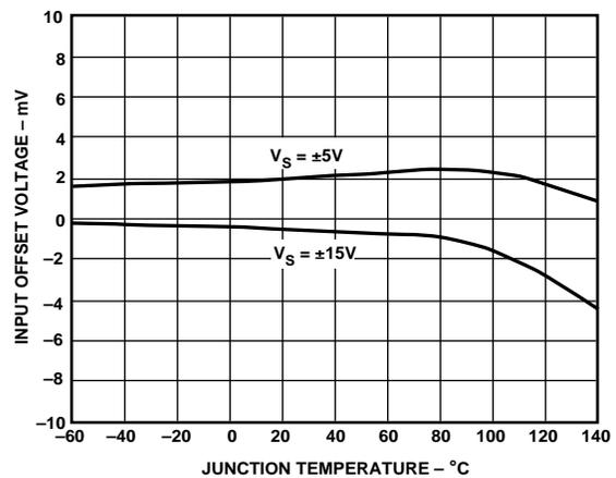
Figure 6. Input Offset Voltage vs. Junction Temperature
