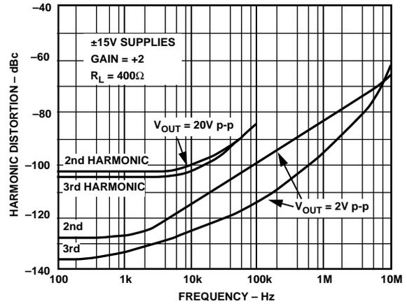
Figure 16. Harmonic Distortion vs. Frequency ( $R_L = 400 \Omega$ )
