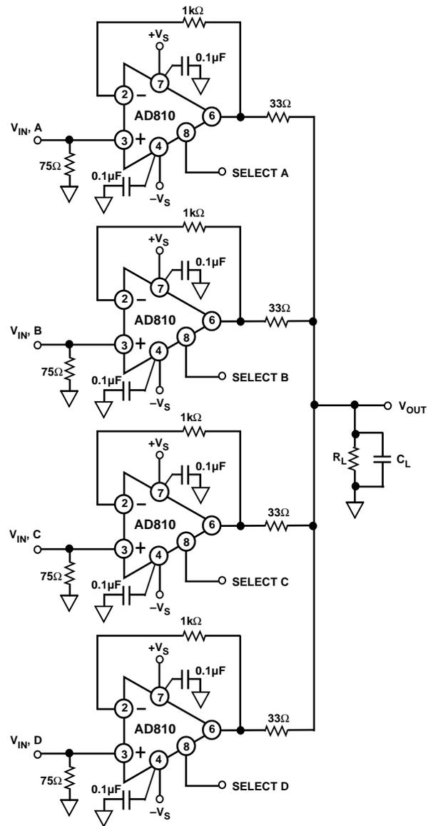
Figure 58. A 4:1 Multiplexer Driving a High Impedance
