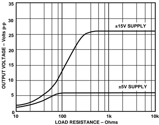
Figure 3. Output Voltage Swing vs. Load Resistance
