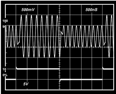
Figure 52. Channel Switching Time for the 2:1 Mux
