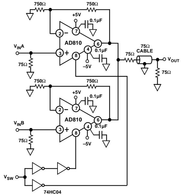
Figure 54. A Fast Switching 2:1 Video Mux
