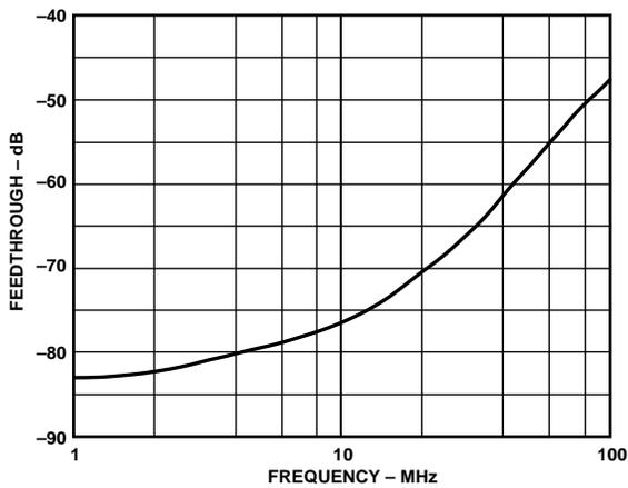
Figure 53. 2:1 Mux OFF Channel Feedthrough vs. Frequency
