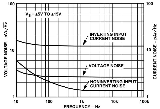
Figure 12. Input Voltage and Current Noise vs. Frequency
