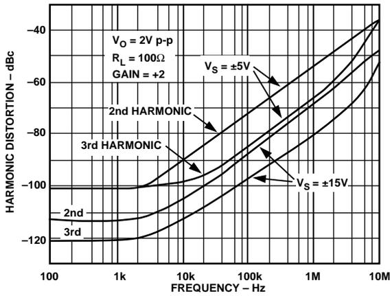
Figure 15. Harmonic Distortion vs. Frequency ( $R_L = 100 \Omega$ )
