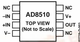
Figure 3. 8-Lead MSOP (RM Suffix)
