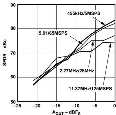
Figure 9. Single-Tone SFDR vs.  $A_{OUT}$  @  $f_{OUT} = f_{CLOCK}/11$
