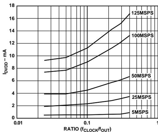
Figure 26.  $I_{DVDD}$  vs. Ratio @  $DVDD = 5\text{ V}$
