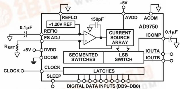
The AD9750 is a current-output DAC with a nominal full-scale output current of 20 mA and > 100 kΩ output impedance.
