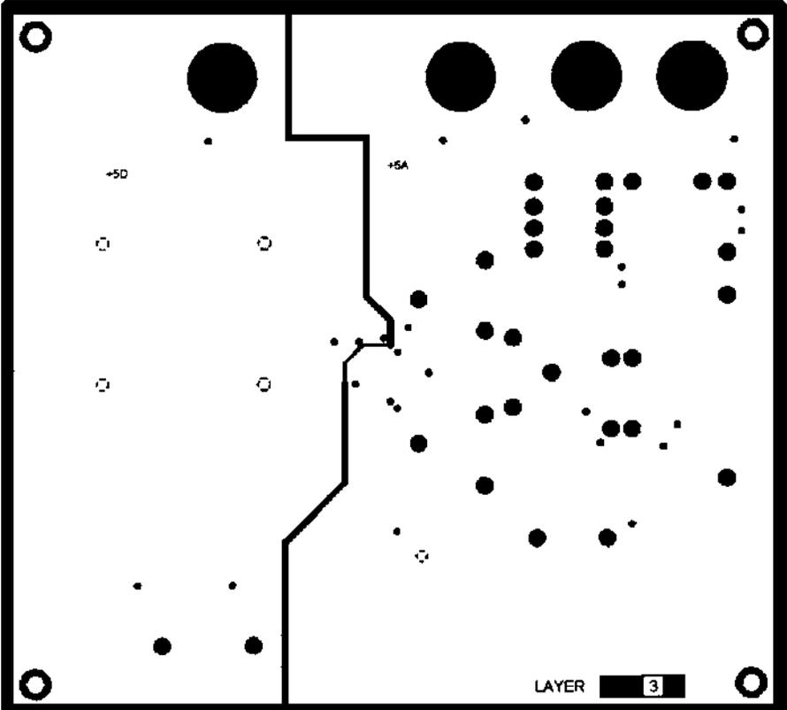
Figure 42. Power Plane PCB Layout (Layer 3)
