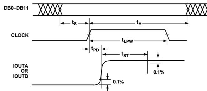
Figure 1. Timing Diagram
