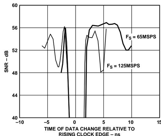
Figure 24. SNR vs. Clock Placement  $2 f_{OUT} = 10 \text{ MHz}$
