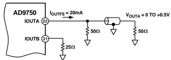
Figure 31. 0 V to +0.5 V Unbuffered Voltage Output
