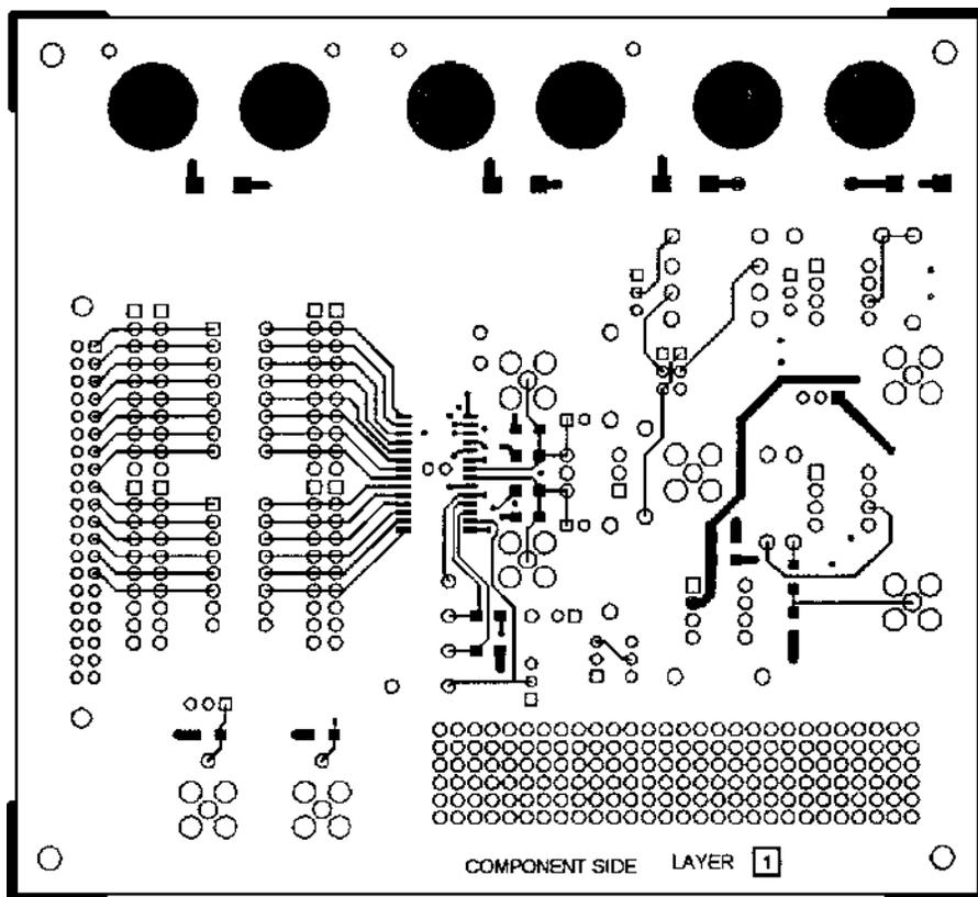
Figure 40. Component Side PCB Layout (Layer 1)
