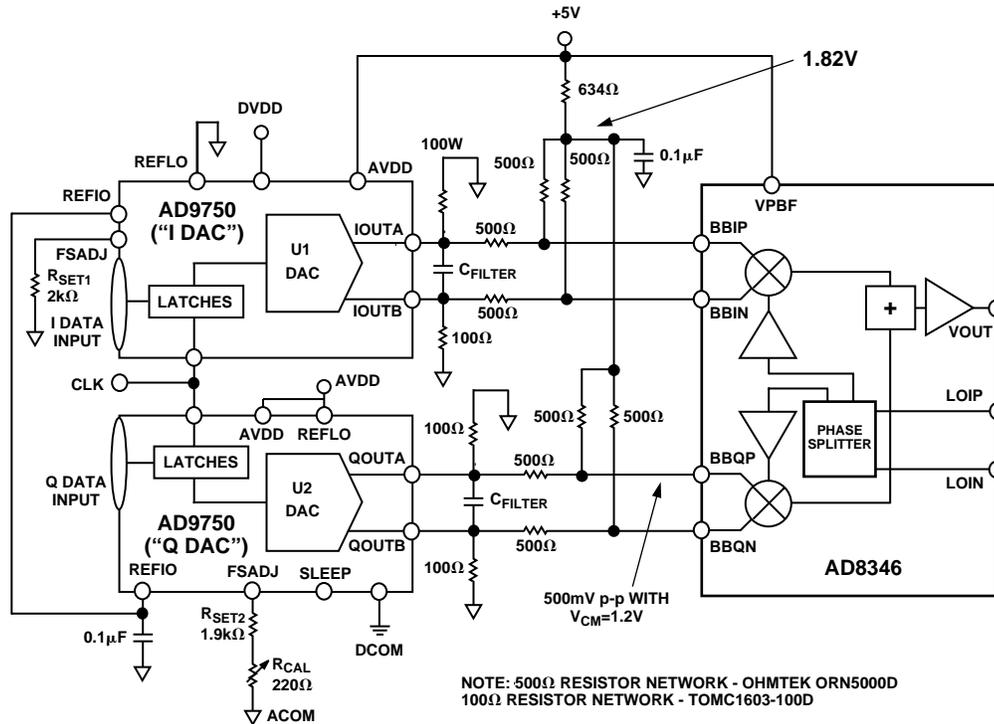
Figure 36. Baseband QAM Implementation Using Two AD9750s
