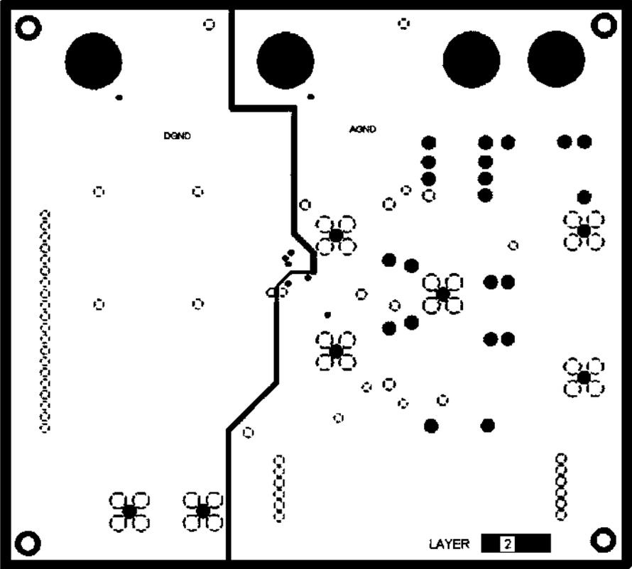
Figure 41. Ground Plane PCB Layout (Layer 2)
