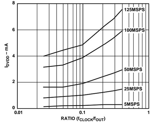
Figure 27.  $I_{DVDD}$  vs. Ratio @  $DVDD = 3\text{ V}$
