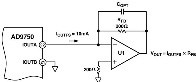
Figure 32. Unipolar Buffered Voltage Output
