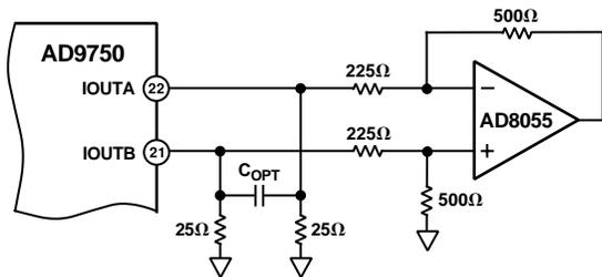
Figure 29. DC Differential Coupling Using an Op Amp
