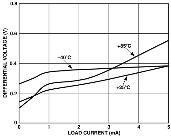
TPC 11. ADR380 Minimum Input/Output Voltage Differential vs. Load Current
