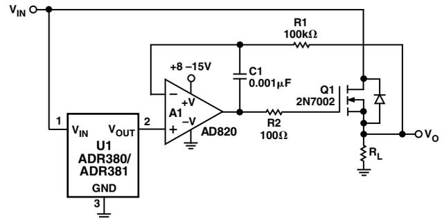
Figure 5. ADR380/ADR381 for Precision High Current Voltage Source
