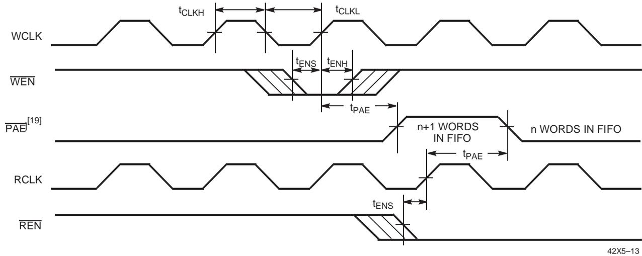
**Programmable Almost Empty Flag Timing (applies only in  $\overline{SMODE}$  ( $\overline{SMODE}$  is LOW))**
