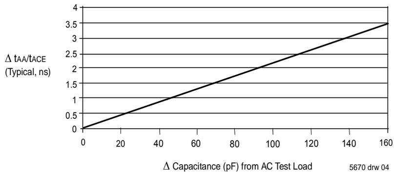
Figure 3. Typical Output Derating (Lumped Capacitive Load).
