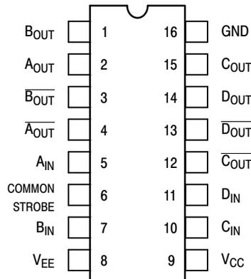
Pin assignment is for Dual-in-Line Package.
