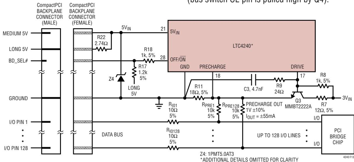
Figure 13. Precharge Application Circuit for 5V Signaling Systems
