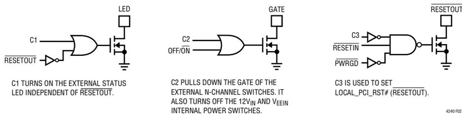
Figure 2. Send Byte Command Latch and Logic
