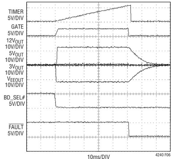
Figure 6. Power-Up into a Short on 3.3V Output
