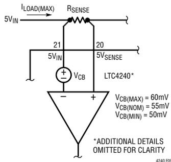
**Figure 9. Circuit Breaker Equivalent Circuit for Calculating  $R_{\text{SENSE}}$**
