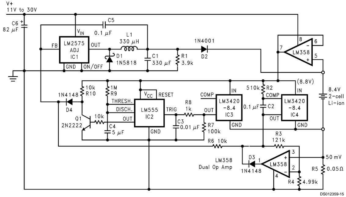
FIGURE 10. (Fast) Pulsed Constant Current 2-Cell Charger
