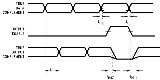
FIGURE 2. Propagation Delay, Cut-Off and Transition Times
