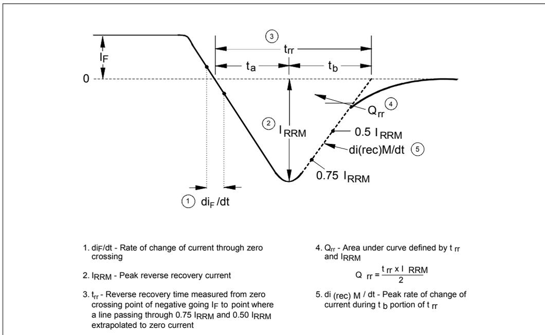
**Fig. 10 - Reverse Recovery Waveform and Definitions**
