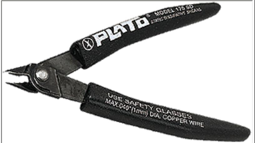
**Platoshear 170 SMD - ESD Safe:** Designed for use in restricted areas. The low profile cutting head width of .290" (7.38mm) and an end radius of .010" (.25mm) is designed to cut between SMD leads as close as .040" (1mm) center to center and up to .025" (0.6mm) in diameter. Includes unique SAF-T-LINK® feature for greater operator safety.
