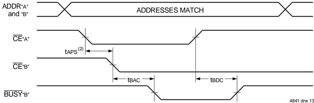
**Waveform of  $\overline{\text{BUSY}}$  Arbitration Cycle Controlled by Address Match Timing ( $M/\overline{\text{S}} = V_{IH}$ )<sup>(1)</sup>**
