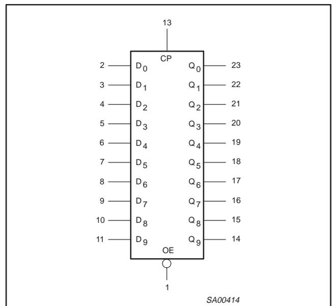
10-bit D-type flip-flop with 5-volt tolerant inputs/outputs; positive-edge trigger (3-State)
