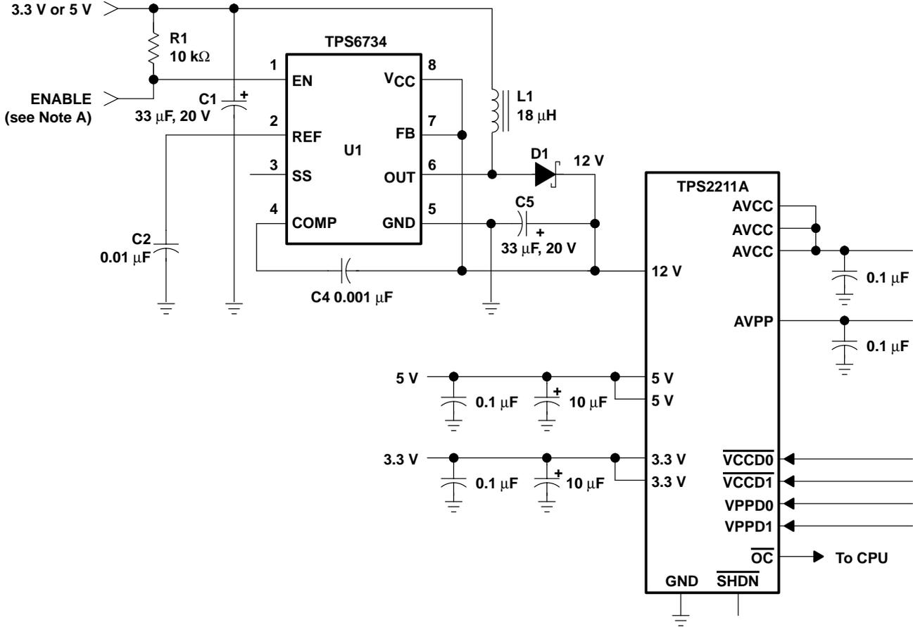
NOTE A: The enable terminal can be tied to a general-purpose I/O terminal on the PCMCIA controller or tied high.
