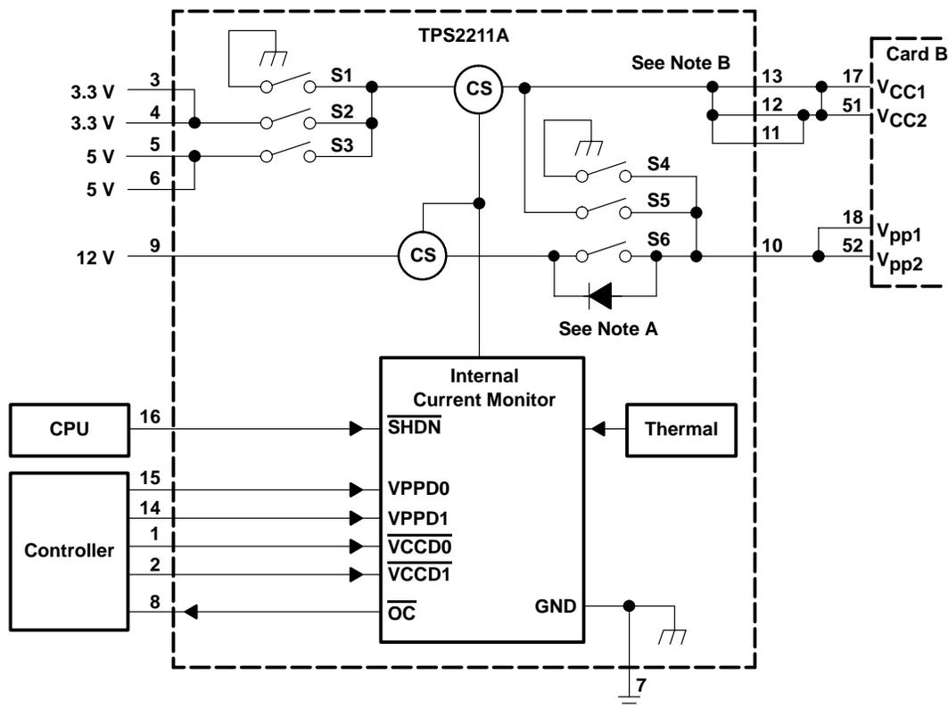
NOTE A: MOSFET switch S6 has a back-gate diode from the source to the drain. Unused switch inputs should never be grounded.
