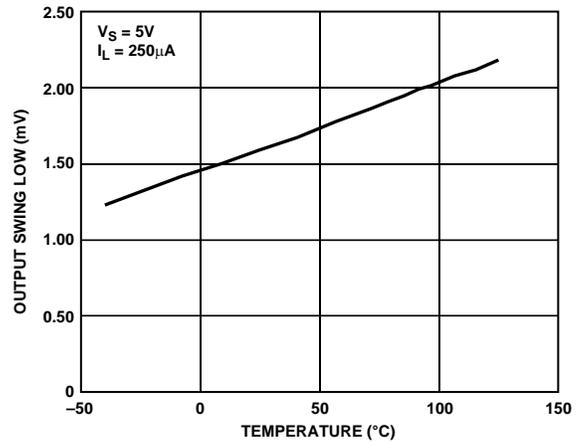
Figure 14. Output Voltage Swing Low vs. Temperature
