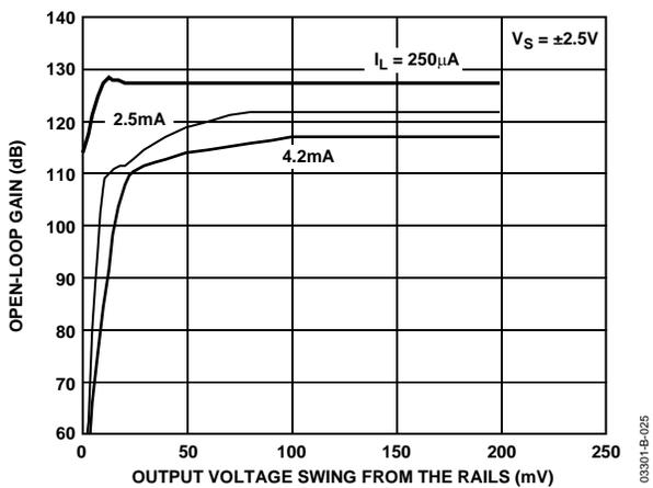
Figure 25. Open-Loop Gain vs. Output Voltage Swing
