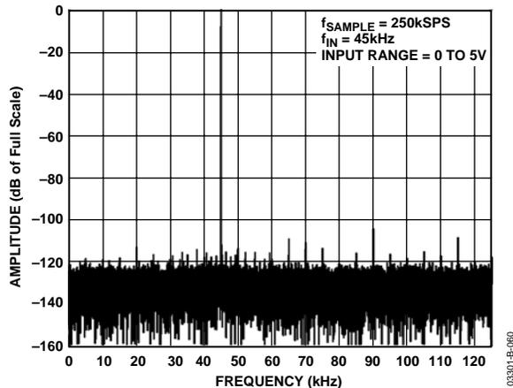
Figure 59. Frequency Response of AD8651 Driving a 16-Bit ADC
