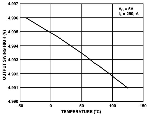
Figure 13. Output Voltage Swing High vs. Temperature
