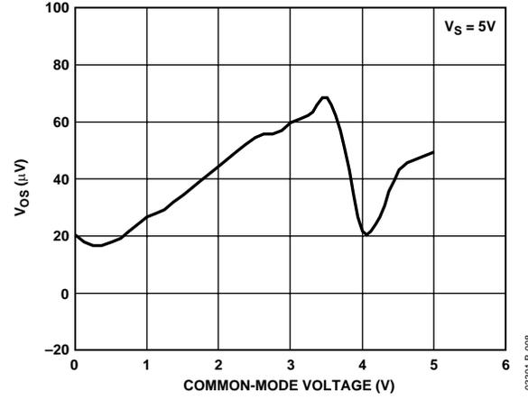
Figure 8. Input Offset Voltage vs. Common-Mode Voltage
