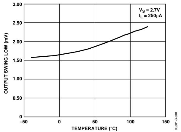
Figure 40. Output Voltage Swing Low vs. Temperature
