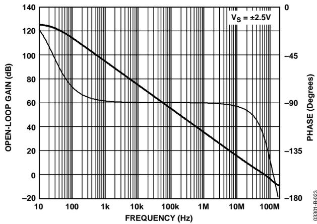
Figure 23. Open-Loop Gain and Phase vs. Frequency
