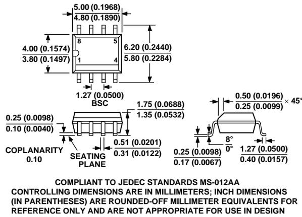
Figure 62. 8-Lead Standard Small Outline Package [SOIC] (R-8)
