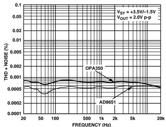
Figure 57. Total Harmonic Distortion
