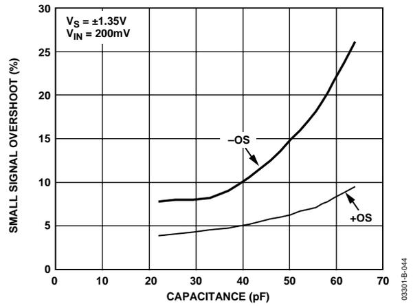
Figure 44. Small Signal Overshoot vs. Load Capacitance
