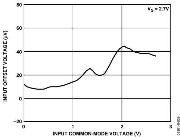
Figure 36. Input Offset Voltage vs. Common-Mode Voltage
