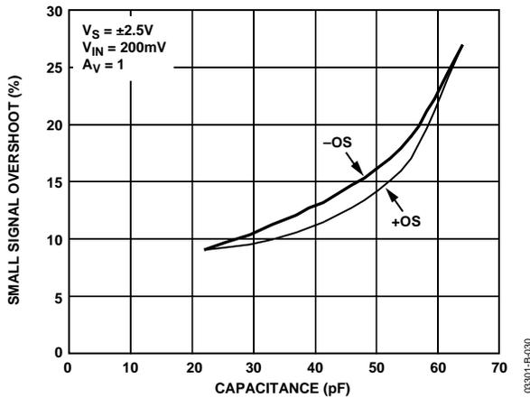
Figure 30. Small Signal Overshoot vs. Load Capacitance
