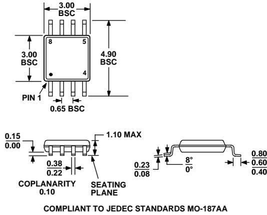
Figure 61. 8-Lead Mini Small Outline Package [MSOP] (RM-8)
