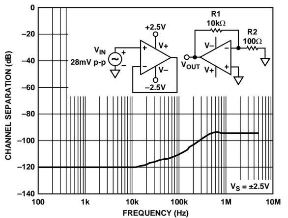
Figure 52. Channel Separation
