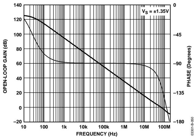
Figure 49. Open-Loop Gain and Phase vs. Frequency
