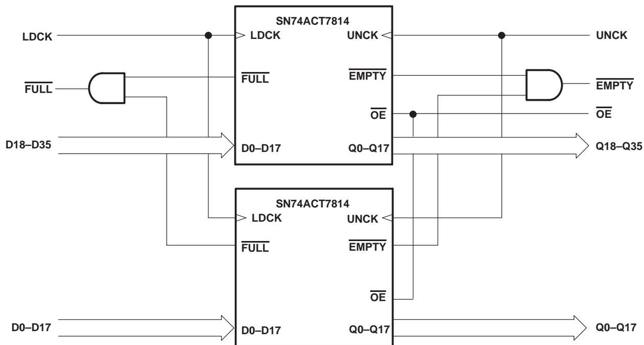
Figure 6. Word-Width Expansion: 64 × 36 Bits
