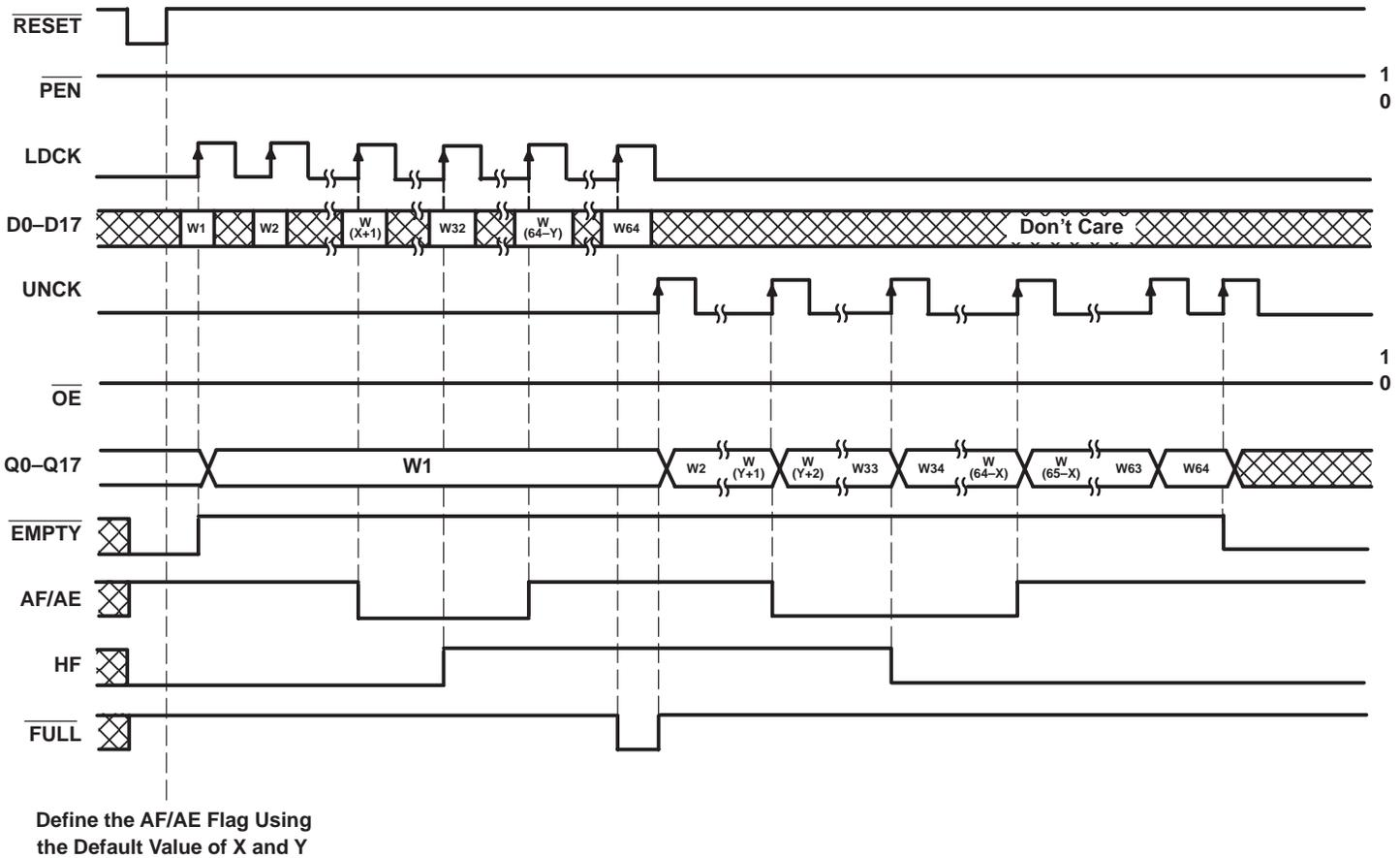
Figure 2. Write, Read, and Flag Timing Reference
