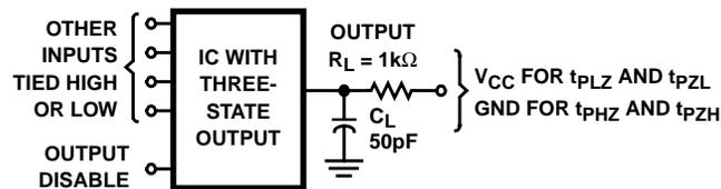
NOTE: Open drain waveforms  $t_{PLZ}$  and  $t_{PZH}$  are the same as those for three-state shown on the left. The test circuit is Output  $R_L = 1k\Omega$  to  $V_{CC}$ ,  $C_L = 50pF$ .
