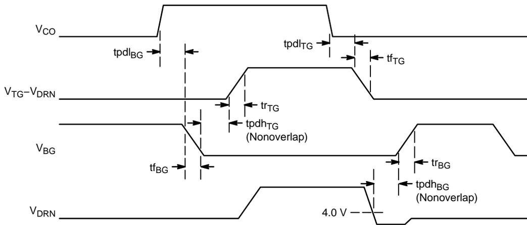
Figure 2. Timing Diagram
