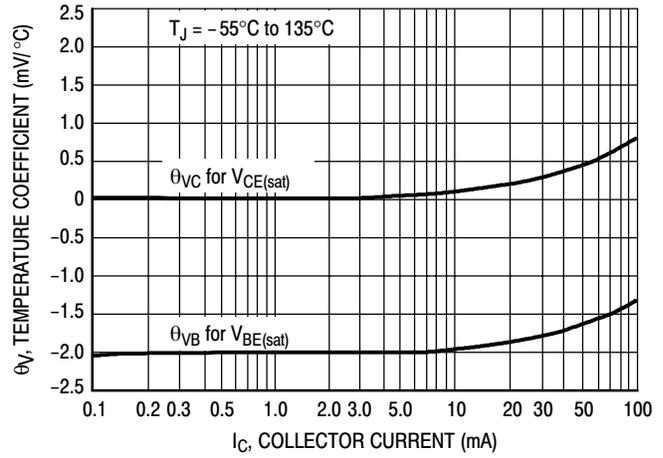
Figure 5. Temperature Coefficients
