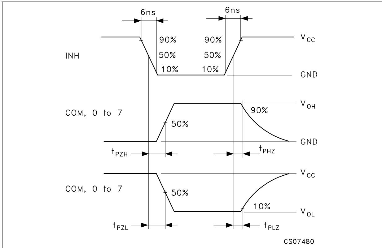
**WAVEFORM: PROPAGATION DELAY (f=1MHz; 50% duty cycle)**
