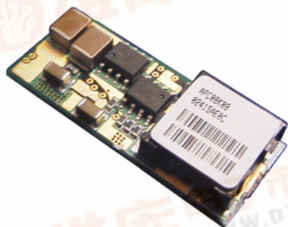
Industry Standard 0.53 X 1.3 X 0.29H SMT Package
