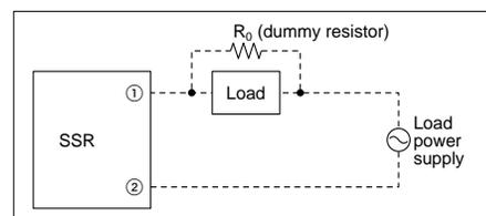
Load specification: AC output type 20 mA
