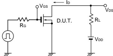
Fig.8 Switching time measurement circuit
