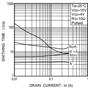
Fig.7 Switching characteristics
