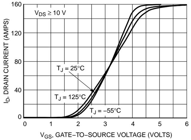
Figure 2. Transfer Characteristics
