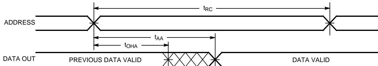
Read Cycle No. 2 ( $\overline{OE}$  Controlled)<sup>[11, 12]</sup>
