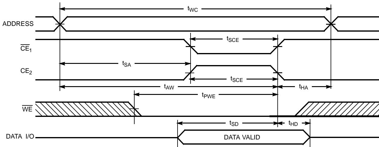
**Write Cycle No. 2 ( $\overline{WE}$  Controlled,  $\overline{OE}$  HIGH During Write)<sup>[13, 14]</sup>**
